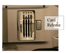
NOTE\* - EACH CAMERA COMES WITH ONLY ONE CARD. PLACE THE CARD IN THE LOWEST NUMBERED SLOT. ADDITIONAL CARDS MAY BE AVAILABLE IF NECESSARY.
