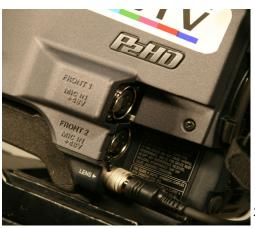
If you do not need the camera mic, be sure to turn the channel not being used by the rear XLR connection to "rear", which will disengage the front mic.
